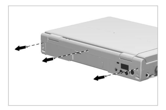
Figure 5-22. Removing the CPU Cover Screws
